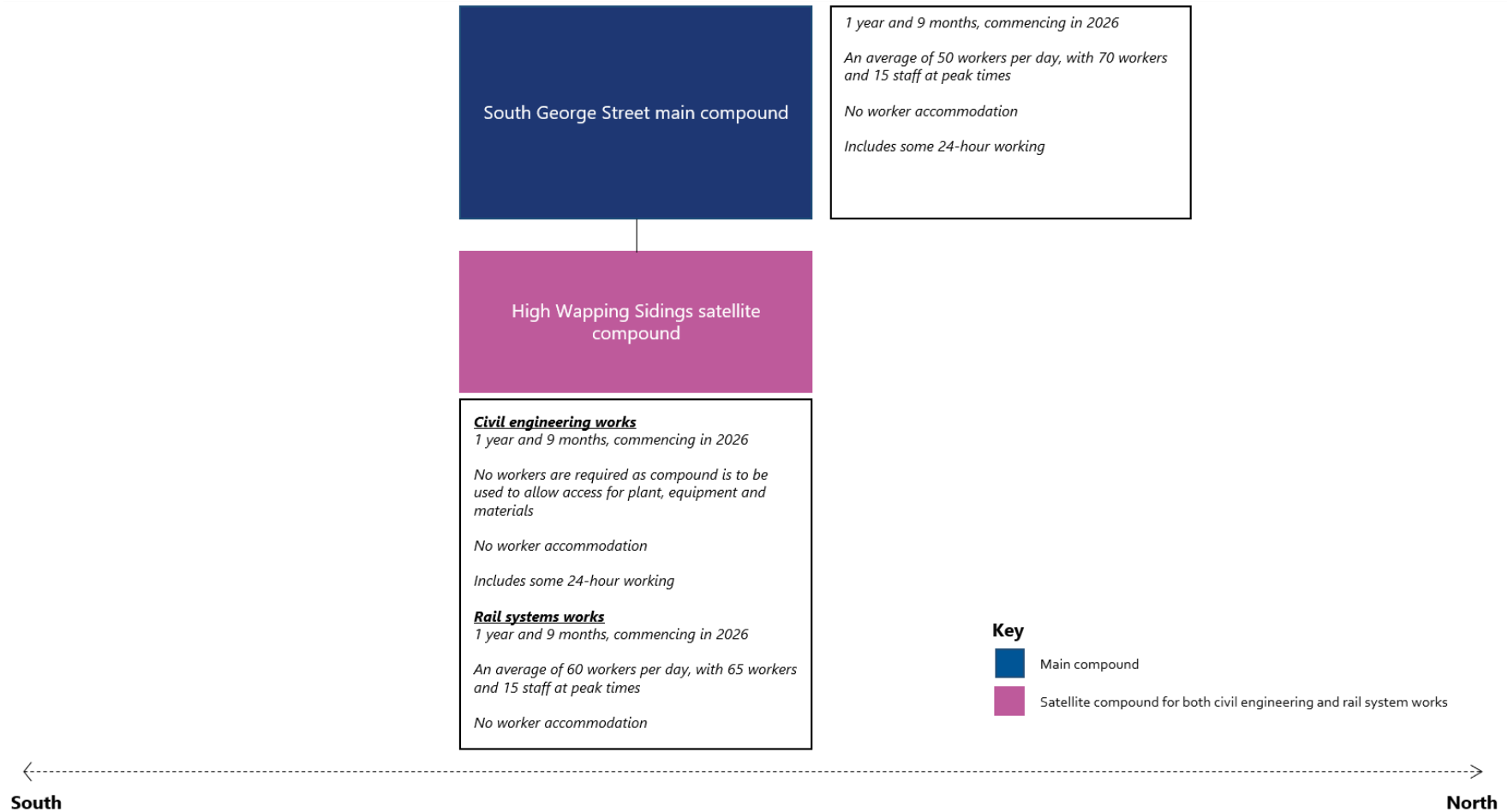
Figure 8: Construction compounds for civil engineering and railway system works
