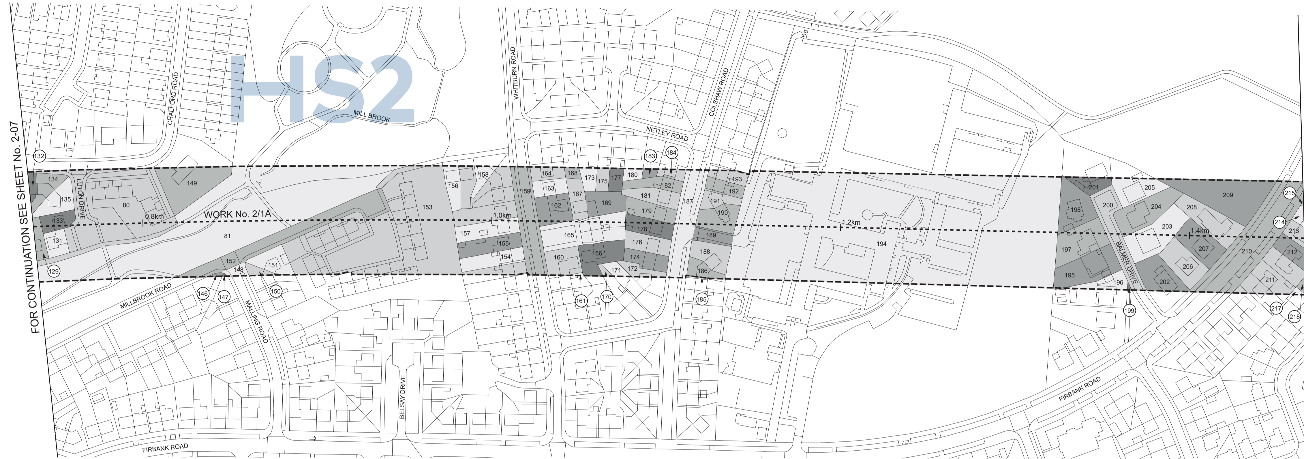
Proposed Tunnel below Mill Brook, Work No. 2/1A, depth of Tunnel below river bed 17.30m.
