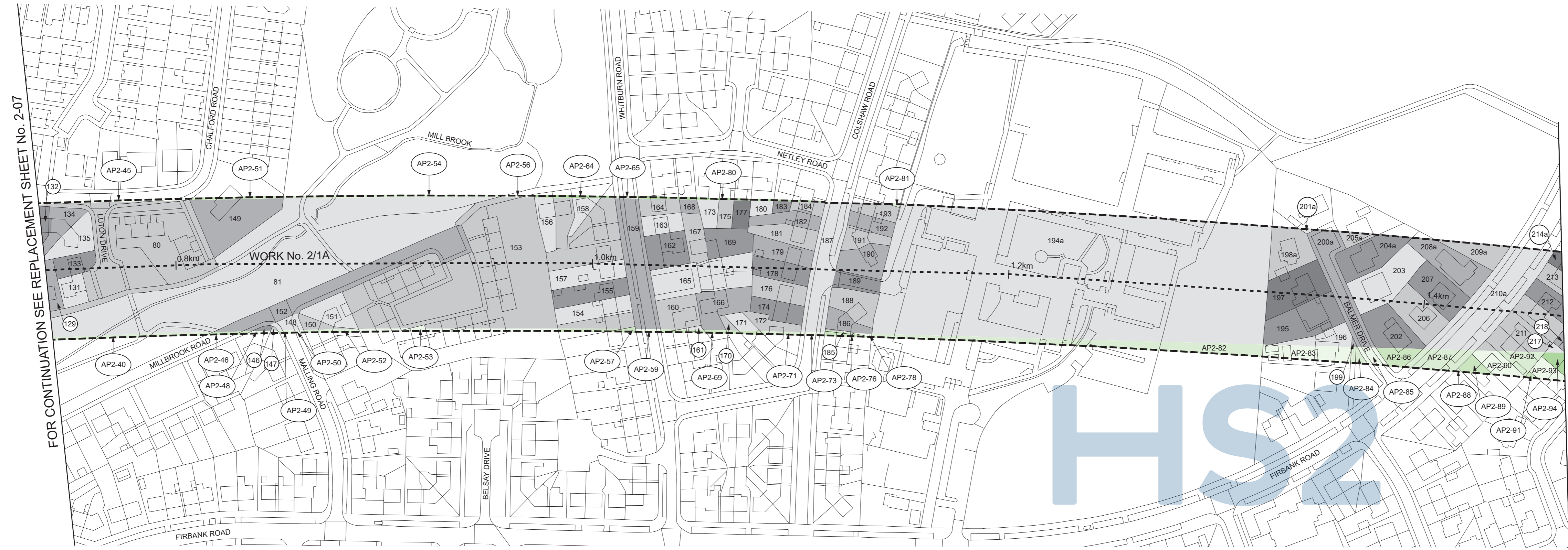
Proposed Tunnel below Mill Brook, Work No. 2/1A, depth of Tunnel below river bed 18.42m.
