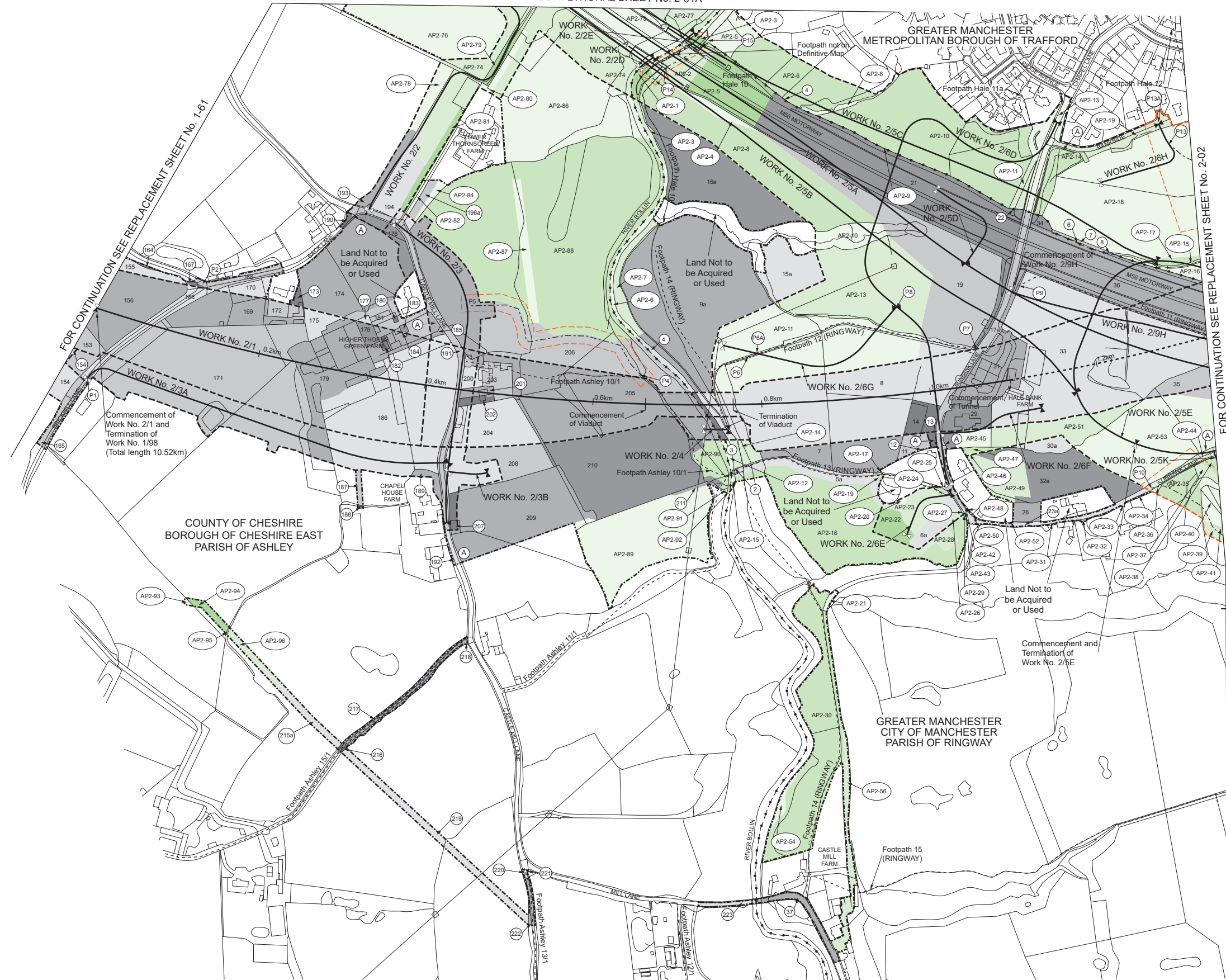
Proposed Bridge over River Bollin, Work No. 2/5A, span 74.27m, headway 9.62m. Proposed Bridge over Tributary of River Bollin, Work No. 2/6D, span 23.50m, headway 19.98m. Proposed Railway over River Bollin, Work No. 2/1, span 32.00m, headway 13.38m. Proposed Temporary Bridge over River Bollin, Work No. 2/4, span 29.25m, headway 6.37m.
